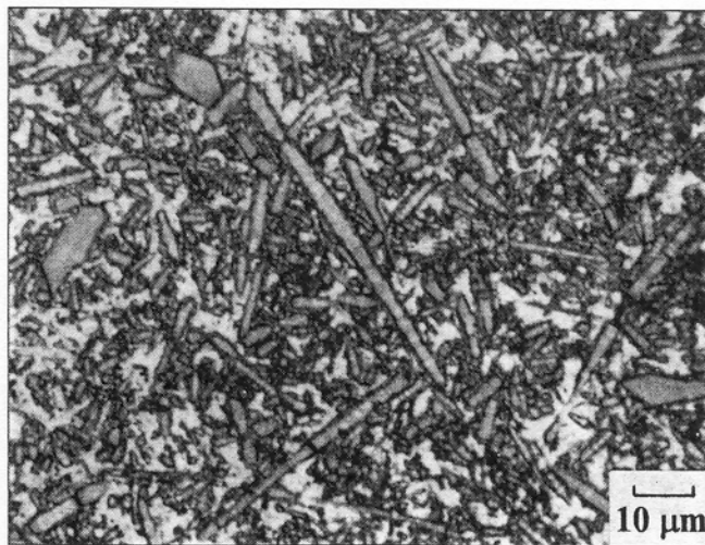
Figure 5. Optical micrograph of polished section of Cu/SiCw composite with 54.5v/o SiCw made by the coated filler method.
